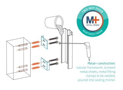
REMARKS: The principle of these section drawings is valid for almost all our surface-mounted swing doors. The standard thickness of the doorleaf is 72 mm. The fireproof doors EI1 60 have a thickness of 82 mm! Other section drawings are available, see: www.heinen-doors.com.
