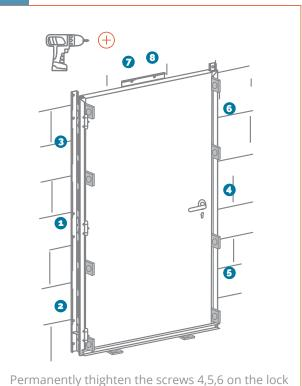
Permanently thighten the screws 4,5,6 on the lock side of the frame and 7 and 8 on the top profile.
