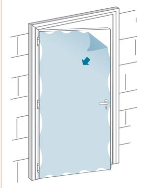
Remove the blue protective film from the leaf and remove any traces of concrete using a damp cloth.
