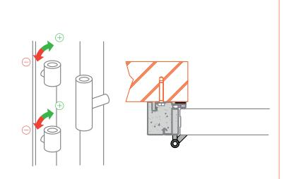
Only adjust the hinge parts of the frame. The compression of the lock surround can be adjusted using the striker plates (see chapter on striker plate adjustment).
