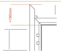
Maintain a free edge of at least 190 mm above the wall opening the wall opening, so that the cover can be clipped on later.
