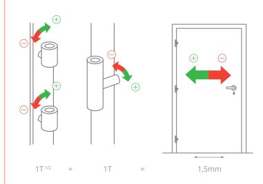
Clockwise: reduces the slack around the hinge.
