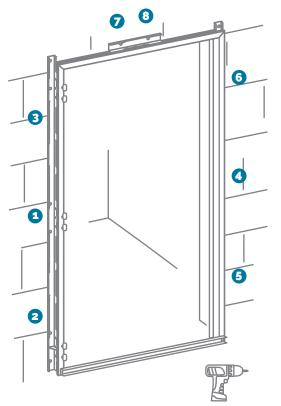
Tighten screws 1, 2 and 3 on the hinge side of the frame slightly tighten screws 4, 5 and 6 on the lock side, as well as slightly tighten screws 7 and 8 on the top profile.
